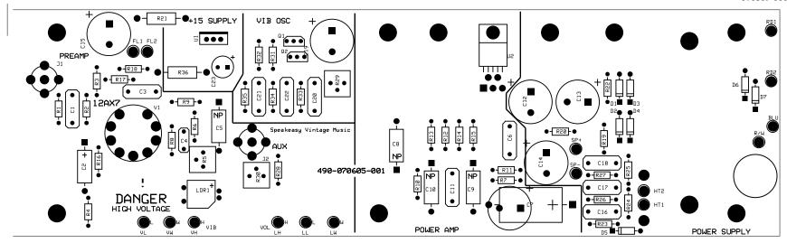
The Volume and Tone control terminals are laid out exactly the same as the original 200 PCB.
